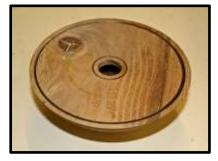
Andy reversed the form in the chuck and trued up the top taking gentle cuts as the piece was hollow and could easily shatter. With a parting tool he removed the plug that was around the screw and cut some decorative rings which he highlighted by burning with the decorative laminate.
